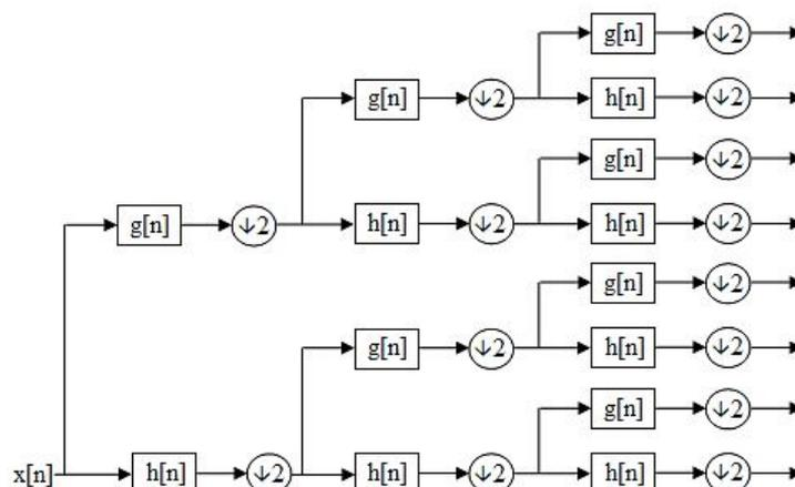
Fig. 3.1: Analysis filter banks for 3 level WPT
